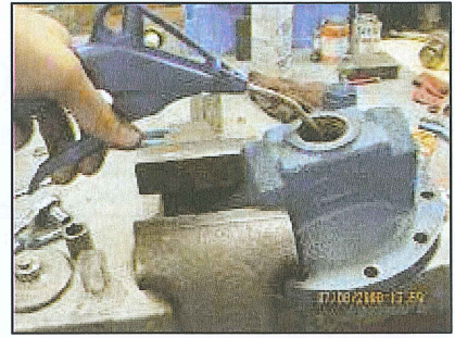
Blow debris from body & reassemble.
