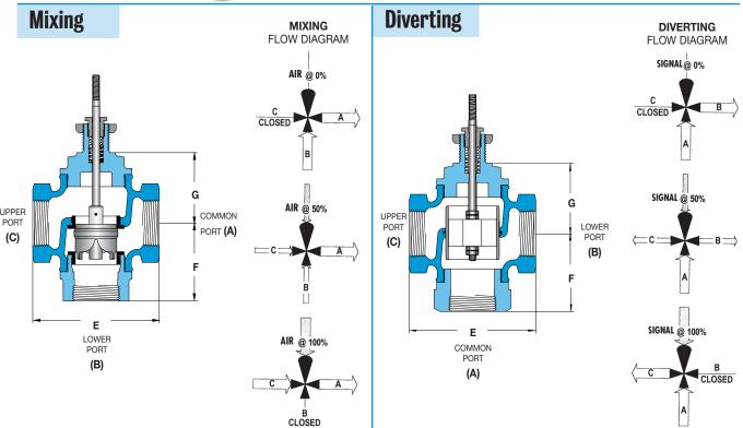
Trerice 3-Way Valves are not designed for use in steam applications. To properly control the mixing of two flows, inlet pressures at ports B and C should be as equal as possible.
