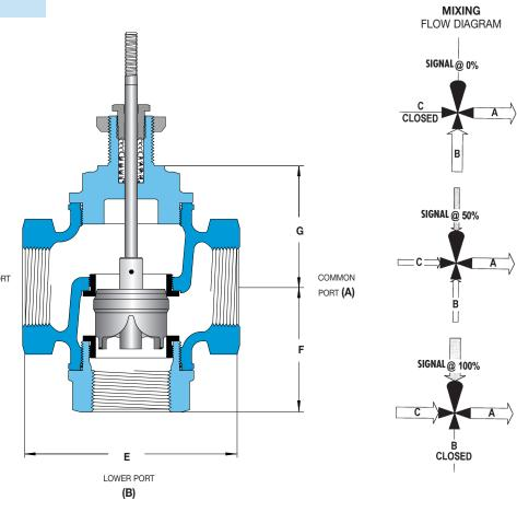
Trerice 3-Way Valves are not designed for use in steam applications.
