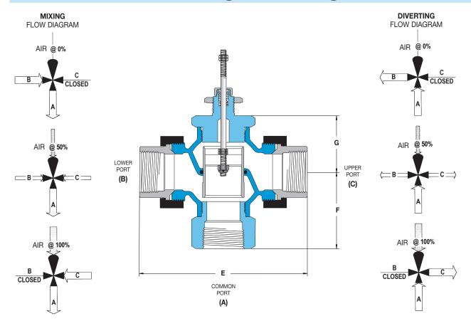
Trerice 3-Way Valves are not designed for use in steam applications.
